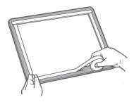
RISO ScreenMaster Mesh and EZIscreen StencilPro films use the same mounting process for each mesh type. Neither mesh is stretched onto the frame as with traditional silk screen mesh - it already has the emulsion attached and therefore is already pre-tensioned and does not require mechanical stretching to a frame. Over stretching the mesh will distort the design and reduce print quality.
