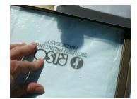
The process involves raising the height of your screen above the item you are printing. The raising of the screen ensures the mesh is not in contact with the item before or after printing and 'snaps' back after the squeegee has passed over the design.
